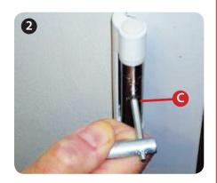
With a 4mm allen key loosen the socket screws (C) by about 1/3 of a turn
