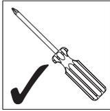
During step 21 the wood screws must be fitted manually using a screwdriver – **DO NOT** use power tools.
