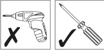
During step **18** the wood screws must be fitted manually using a screwdriver – **DO NOT** use power tools.
