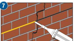
Squeeze the trigger to release the grout and fill the entire length of each slot, ensuring there are no breaks in the bead of grout.
