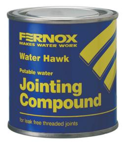
Water Hawk is a pipe jointing compound designed for use with hot and cold potable water. It is suitable for potable water, Natural Gas, steam, air (excluding medical lines) brine, alcohol and L.P. Gas. It is ideal for use on pipe diameters up to 25mm and with reinforcement fibre on pipework over 25mm. The non-toxic formulation is also WRAS approved.
