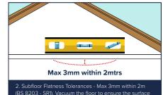
(BS 8203 - SR). Vacuum the floor to ensure the surface is free from debris. Can be used with In-floor Radiant underfloor heating. Source must be min 13mm below flooring. Max Operating floor temperature 29°C refer to instruction manual.
