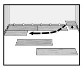
Attach the second plank by connecting the long side to the first row and sliding it up to the short end of the first plank. Check that the long joints of the planks are properly engaged and then press the short joint into place with your fingers.
