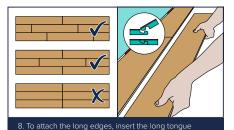
a) to addr the long groupes, insert the long tongue side into the long groupes side of the previous piece at an angle of around 30°. Gently apply inwards and downwards pressure until the joint closes, ensure that the short end joints are accurately aligned. The Plank can then be pushed / tapped flat to lock the joints into place. Always ensure the joints are staggered by at least a third.
