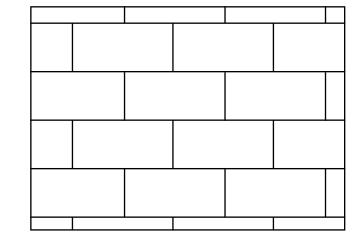
Tile must be installed in a brick pattern, where the seams are staggered.
