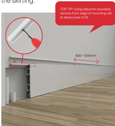
Mounting rail should be clicked onto the skirting, Also securing to the wall using appropriate fixing every 600-1000mm.
