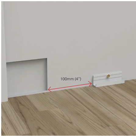
Install the feet 100mm from the start of the skirting.
