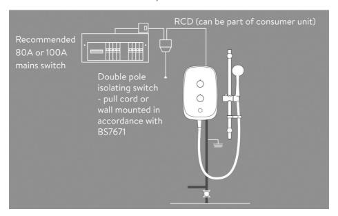
If the consumer unit has a rating below 80A or if there is no spare fuse way, then the installation will not be straightforward.
