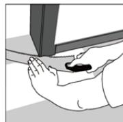
Lay a board (with the decorative side down) next to the door molding and as shown in the figure. Then slide the floorboard under molding.
