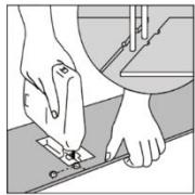
Measure the diameter of the pipe and drill a hole that is 7/8" (20mm) larger. Saw off a piece and lay the board in place on the floor. Then lay the sawed-off piece in place.
