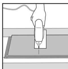
4. **Starting second row:** Rows can be started with end cuts if the cut plank is at least 12" / 30 cm long. If end cut is used for subsequent row a stair step pattern is established. Starting planks of random lengths will create a more aesthetic random stagger. Short end joints must not be closer than 8" / 20 cm to each other.
