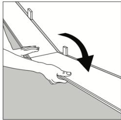
3. **At the end of the first row:** Leave a gap of  $\frac{1}{2}$ " / 10 mm to the wall to avoid any damage while
