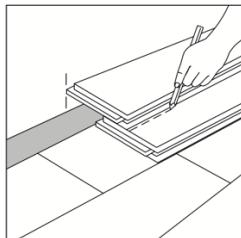
7. **Holes for pipes:** Measure the diameter of the pipe and drill a hole that is  $\frac{3}{4}$ " / 20 mm larger. Saw off a piece as shown in the figure and lay the board in place on the floor. Then lay the sawed-off piece in place.
