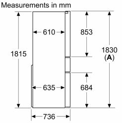
A: Front is adjustable from 1830 to 1847 mm, with front levelling feet fully extended
