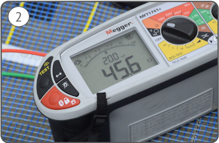
This makes sure no accidental damage has been caused during the cut-and-roll process.
