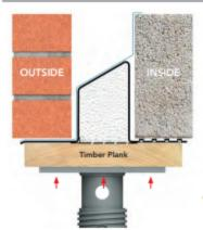
The practice of propping a lintel is sometimes used to facilitate speed of construction. It should only be introduced after initial masonry load has been applied to the lintel.
