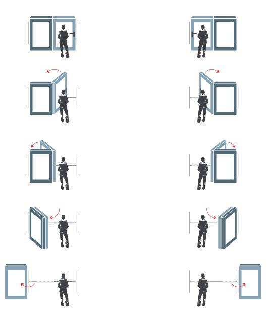
Outer frame can be rotated 180 degrees upon install to allow the doors to be opened towards or away from you depending on your preference.
