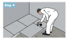
Nine screws per board evenly distributed with a minimum distance from the board edge of 15mm.
