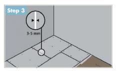
Leave a gap of 3–5mm between each board and screw Knauf AQUAPANEL® Cement Board Floor Tile Underlay to the subfloor using Knauf AQUAPANEL® Maxi Screws SN 25.
