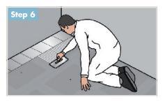
of flexible tile adhesive (class C2/S1 acc. EN 12004/12002), in accordance with manufacturer's guidelines.
