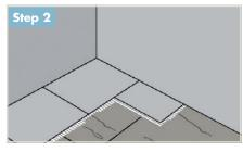
Lay Knauf AQUAPANEL® Cement Board Floor Tile Underlay, starting in the corner farthest from the door. Joints between boards and the subfloor should be staggered (minimum 200mm). No two joints should coincide.
