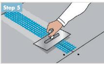
Fill all the joints with flexible tile adhesive Ready to lay tiles: apply a complete bed (class C2/S1 acc. EN 12004/12002), then embed Knauf AQUAPANEL® Tape (10cm). Allow for the adhesive in the joints to dry.
