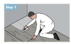
Apply a complete bed of flexible tile adhesive (class C2/S1 acc. EN 12004 (12002) to the subfloor, in accordance with manufacturer's guidelines.Wooden subfloor must be primed before applying Knauf AQUAPANEL® Cement Board Floor Tile Underlay.
