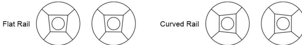
4. Align the Bracket Stems with the Bracket Bases and push the towel rail back into position.
