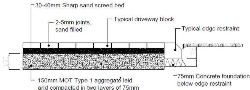
6 Typical section through a driveway constructed in accordance with Marshalls Register Installation Procedures
