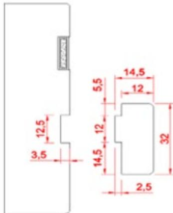
The tongued in stop and grooved frame linings are to comply with the material and dimensional requirements stated within the table in section 3 of the Data Sheet.
