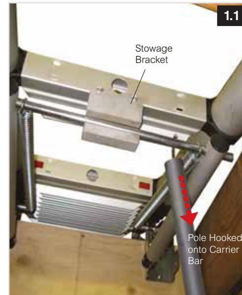
**1.2** Pass the plain end of the pole through the hole in rung 1 and rung 2. Push the pole up to un-hook the ladder stowage bracket on the rear of rung 1 from the sub-frame carrier bar and carefully lower the ladder.
