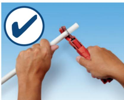
Figure 7: Don't use a hacksaw to cut Hep<sub>2</sub>O pipe
