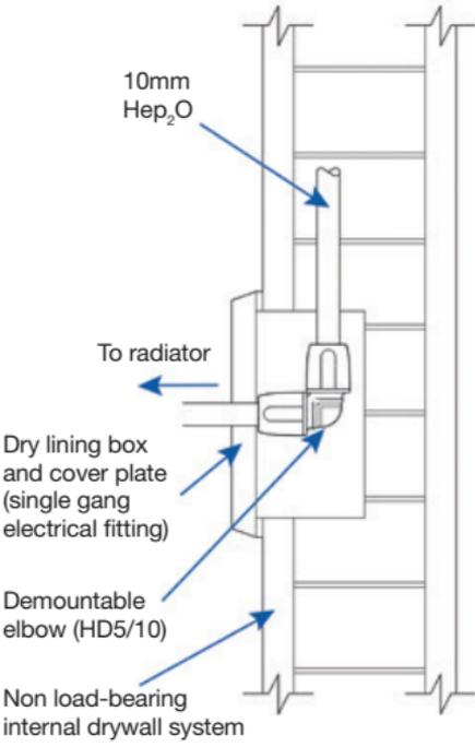
**Note:** This solution can also be used where the radiator is fed from below in which case the risers should be located directly under each box.
