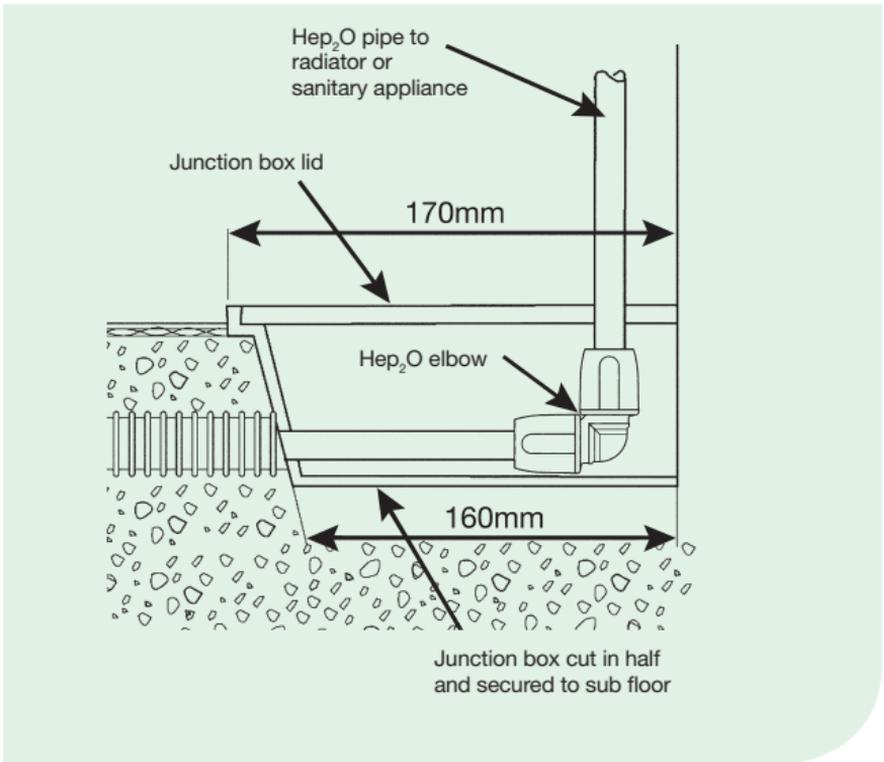
The junction box should be drilled using a hole cutter or spade bit, to allow the conduit to fit snugly and click into position.
