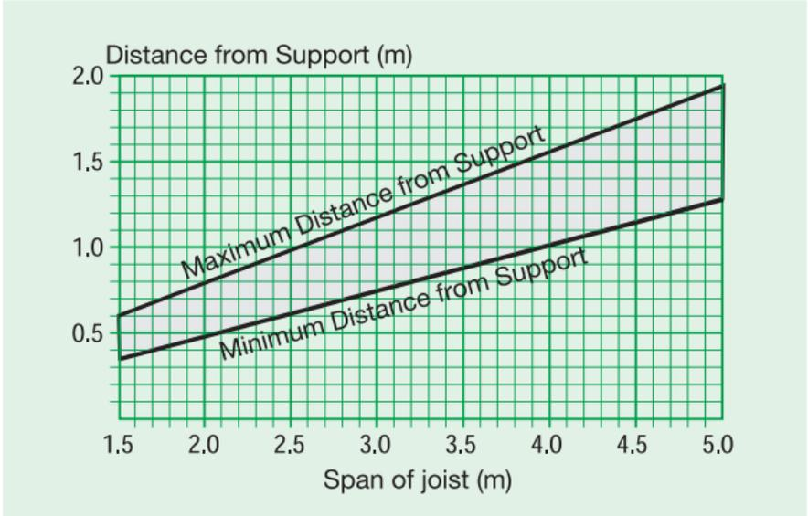
**Note:** This graph should be used in conjunction with Figure 31. **Example of use:** Joist span is 4.5m. Find value on horizontal scale and read up to sloping line. Transfer point of intersection to the vertical scale and read 1.8m.
