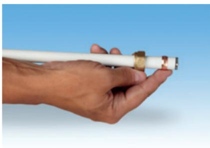
Insert support sleeve into pipe
