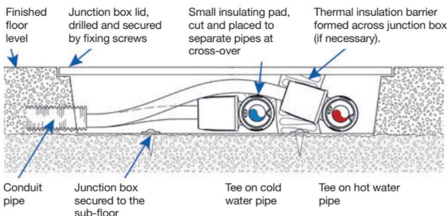
**Note:** Thermal pipe insulation is not necessary when the junction box is used solely for central heating pipes.
