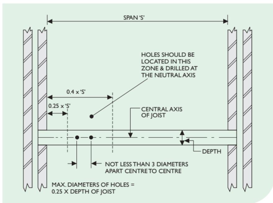
**Note: The minimum distance between a hole and a notch in the same joist should not be less than 100mm.**
