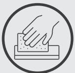
4. After fitting, sand using a 240 grade sand paper, ensuring that all areas of the door are sanded evenly. This provides a “key” to ensure that any subsequent coatings adhere to the pre primed surface efficiently. **Do not apply coatings to the door without sanding the door first.**
