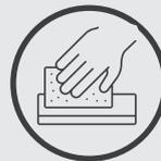
8. After the drying process another light sand of the coating is required using 240 or 320 grade sandpaper. This is to ensure that the second coat adheres to the first.
