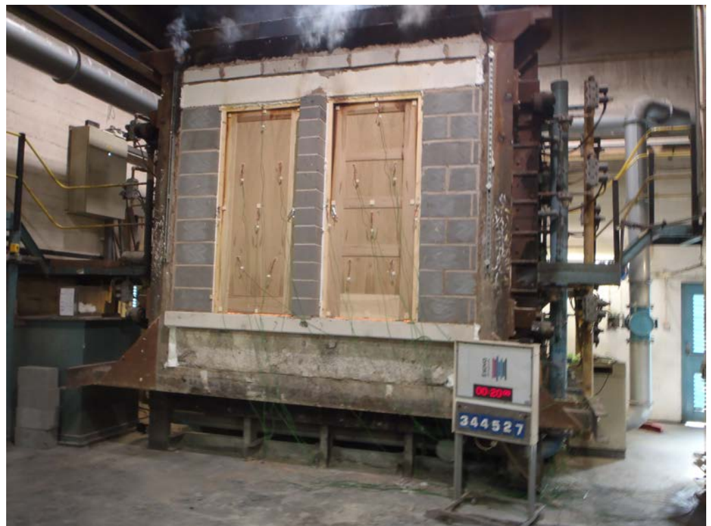
The unexposed face of the test specimens after a test duration of 20 minutes
