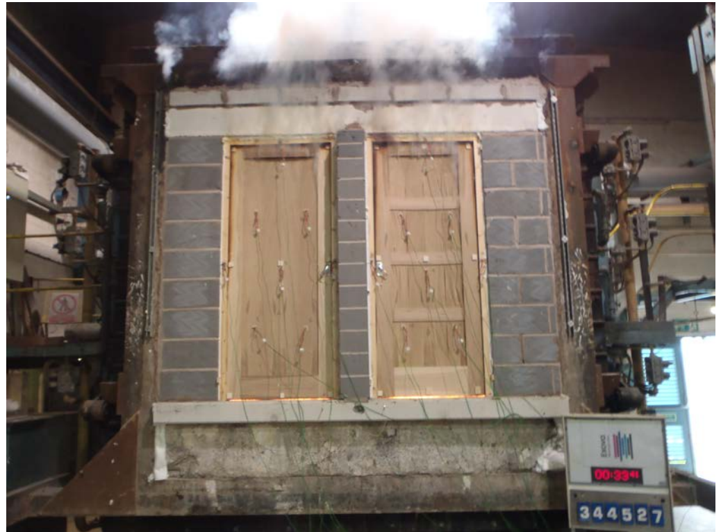
The unexposed face of the test specimens after a test duration of 33 minutes
