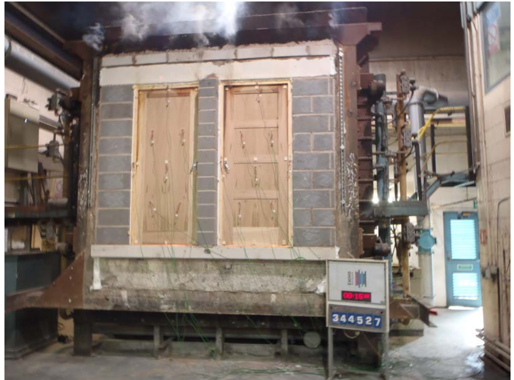
The unexposed face of the test specimens after a test duration of 15 minutes
