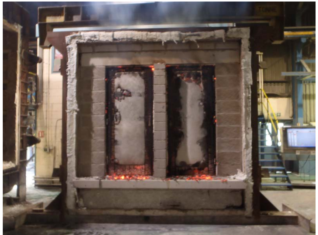
The exposed face of the test specimens after the test
