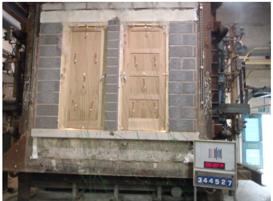
The unexposed face of the test specimens after a test duration of 7 minutes
